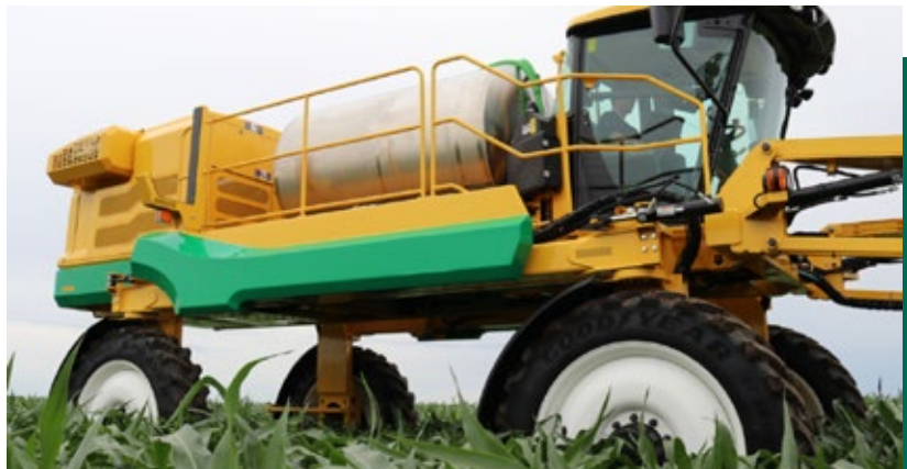
Sprayer made with thermoformed plastic components
